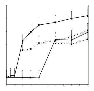
Volume electrical conductivity of PMMA/CNF composites. Results from materials mixed in chaotic mixer and Brabender Plasticorder are identified. ( , 38, 983-993.)
